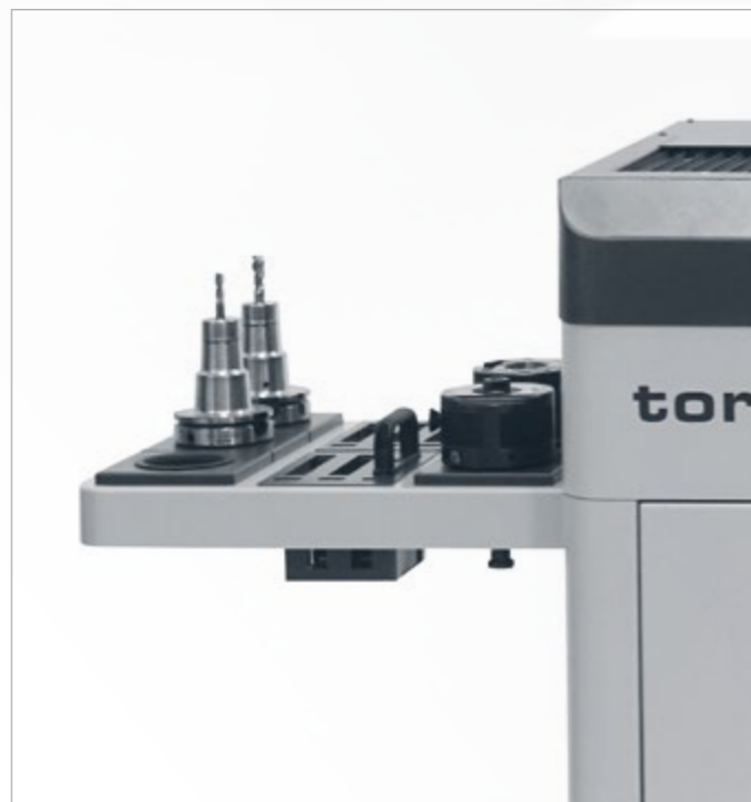
The adapter plates are stored within reach and directly on the machine using a specialized holder.
