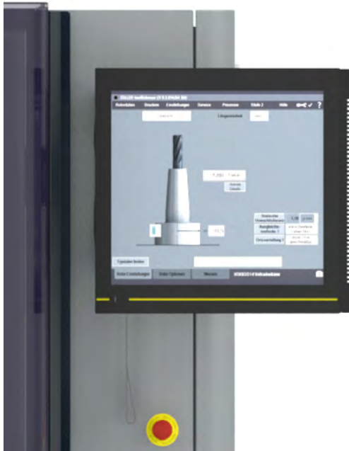
Measuring machine control with ZOLLER operating software on »toolBalancer« with monitor bracket
