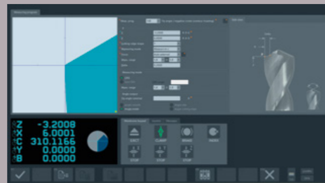
Point angle with hollow grinding – is determined on drilling tools and hollow-ground tool cutting edges from the starting point (outside diameter) to the tool tip or the defined end point by contour tracking.
