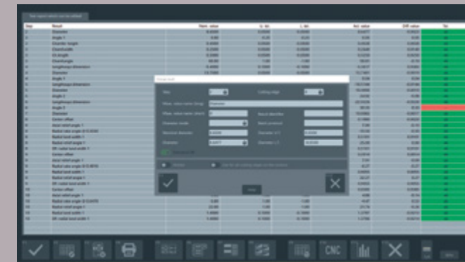
Editable inspection report »apus« – to display all measurement results including designations, nominal values, tolerances and much more in tabular form and flexibly in the layout.
