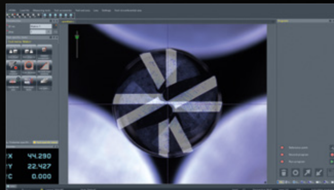
Position the tool to be measured in relation to the reference image
