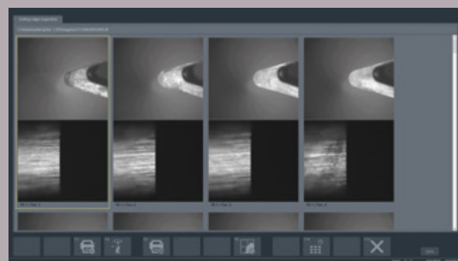
Measuring program 482 – Overview of the recorded cutting edge images including measuring function for determining wear.
