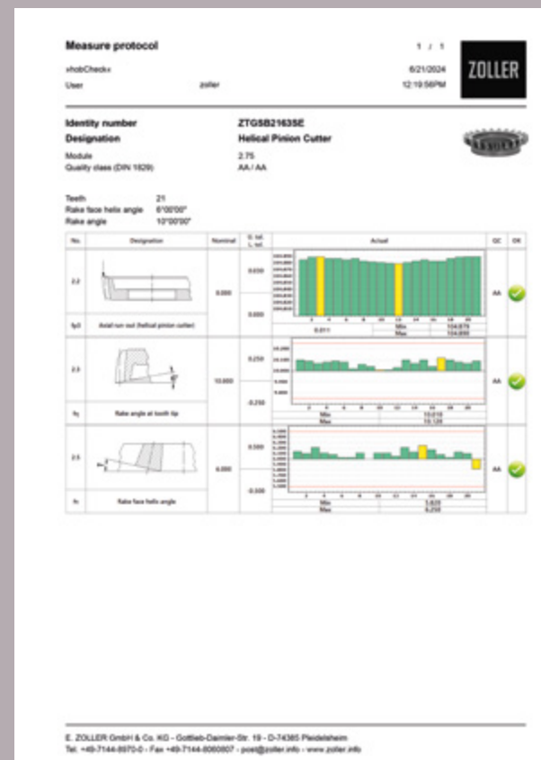
Representative inspection report – including parameter selection for internal and external use.
