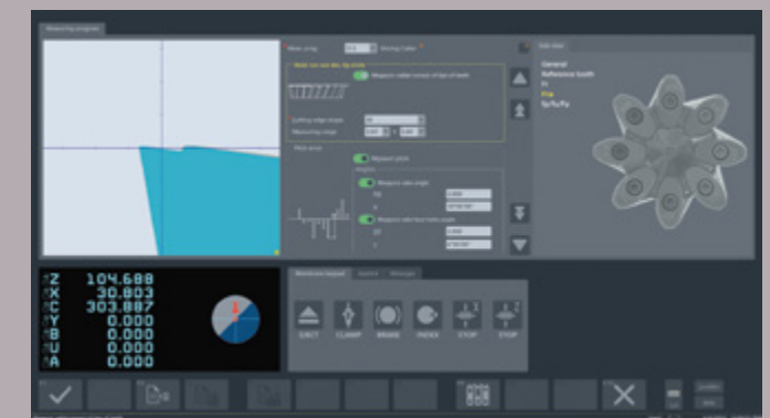
Measuring program 512 – Data creation in the photo-realistic input dialog »fored«.
