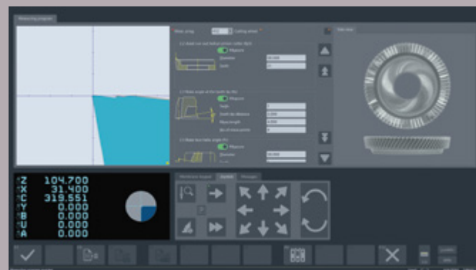
Measuring program 412 – Data creation in the photo-realistic input dialog »fored«.
