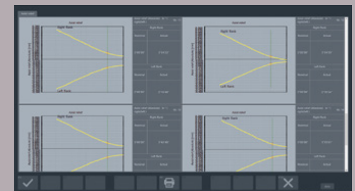
Measuring program 720 – Result display of all measured undercuts as measured values and graphics including zoom function for a detailed analysis.
