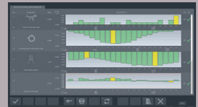
Measuring program 512 – Results display with detailed information for each parameter and re-measurement function.
