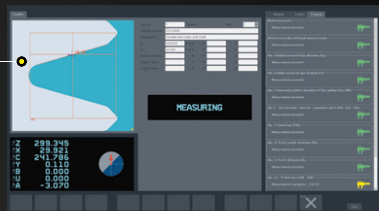
Fully automatic and time-saving measurement with transmitted and incident light image processing and measuring probe
