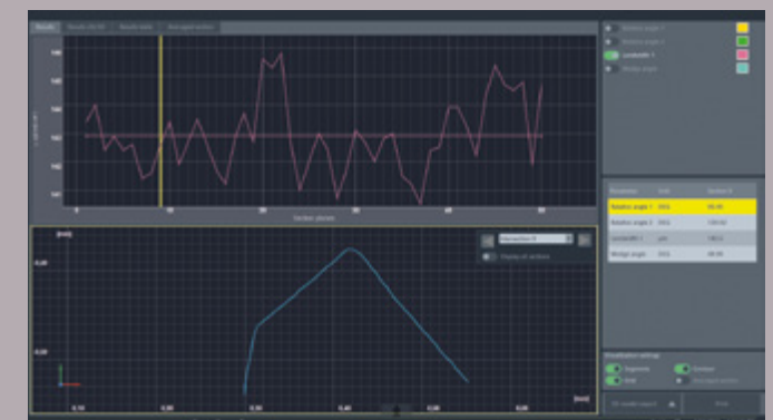
Cutting edge preparation – graphical display of the results across all cutting planes and detailed display of the selected cutting plane.
