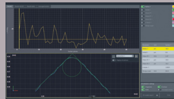
Cutting edge preparation – graphical display of the results across all cutting planes and detailed display of the selected cutting plane.
