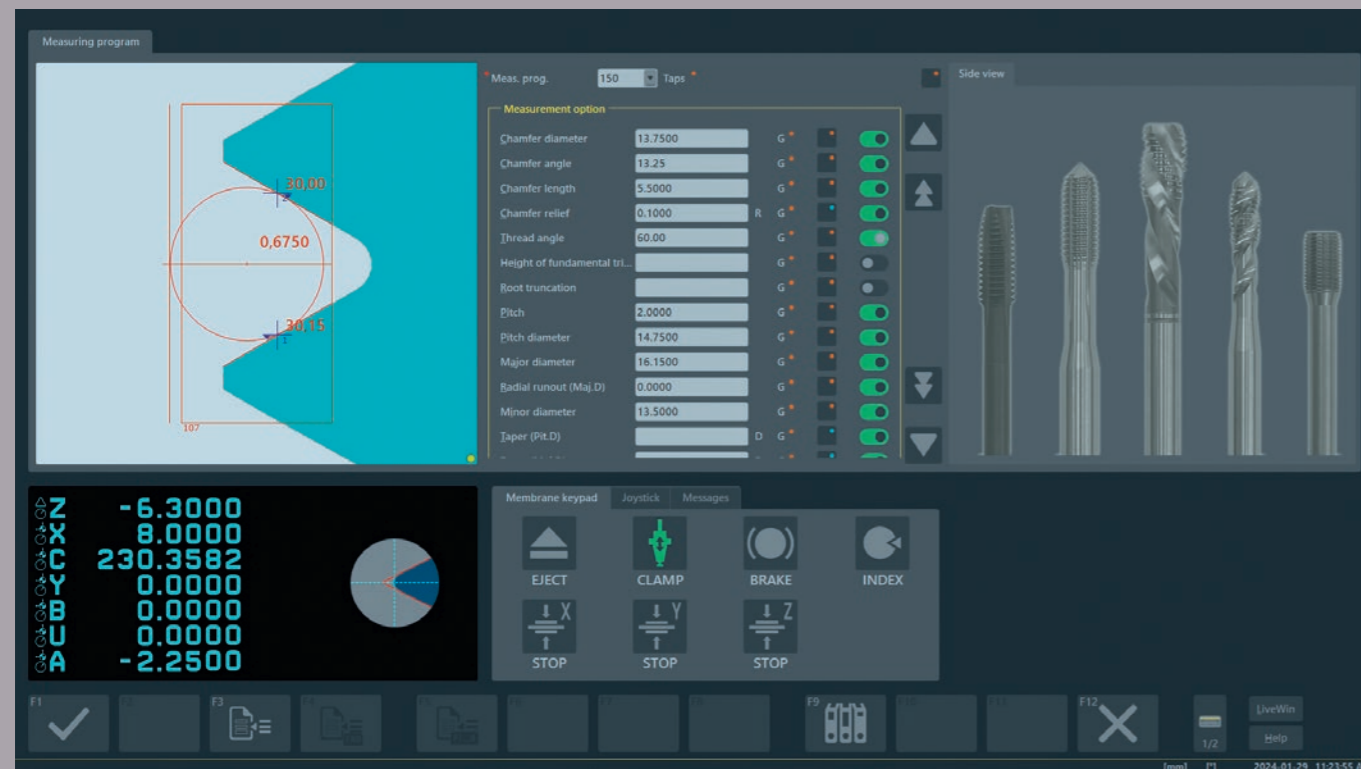
ZOLLER thread measuring program – for metric ISO, ANSI and Whitworth pipe threads
