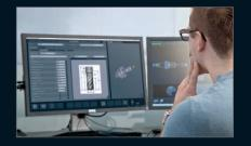
Generation of the measuring sequence at the external workstation using the software module »caz« which simulates a measuring machine.
