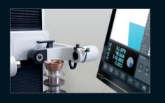
Measuring the grinding wheel pack with the ZOLLER measuring machine leads to µm-accurate, centrally stored data for the subsequent process.
