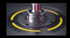
The balancing adapter with center offset is designed with a two-point contact and a pressure element. These features enable a large and more measurable sensor signal.
