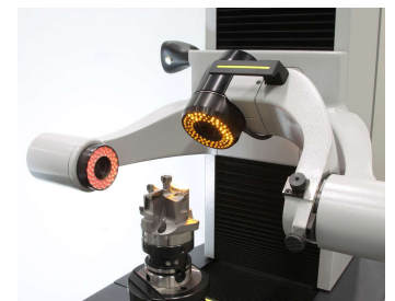
Image 03: With the high-quality, industry-standard »smartCheck« measures tool geometries on the outer contour in transmitted light automatically and with \mu -precision. Manual measurements can be carried out in incident light – even automated using innovative software packages. The high-resolution cutting edge images are ideal for documentation.
